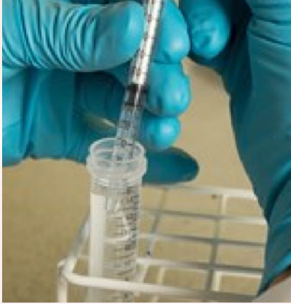
Picture 1: Fill 1 ml syringe with 200 \mu l air, 200 \mu l fish water, 200 \mu l air.
